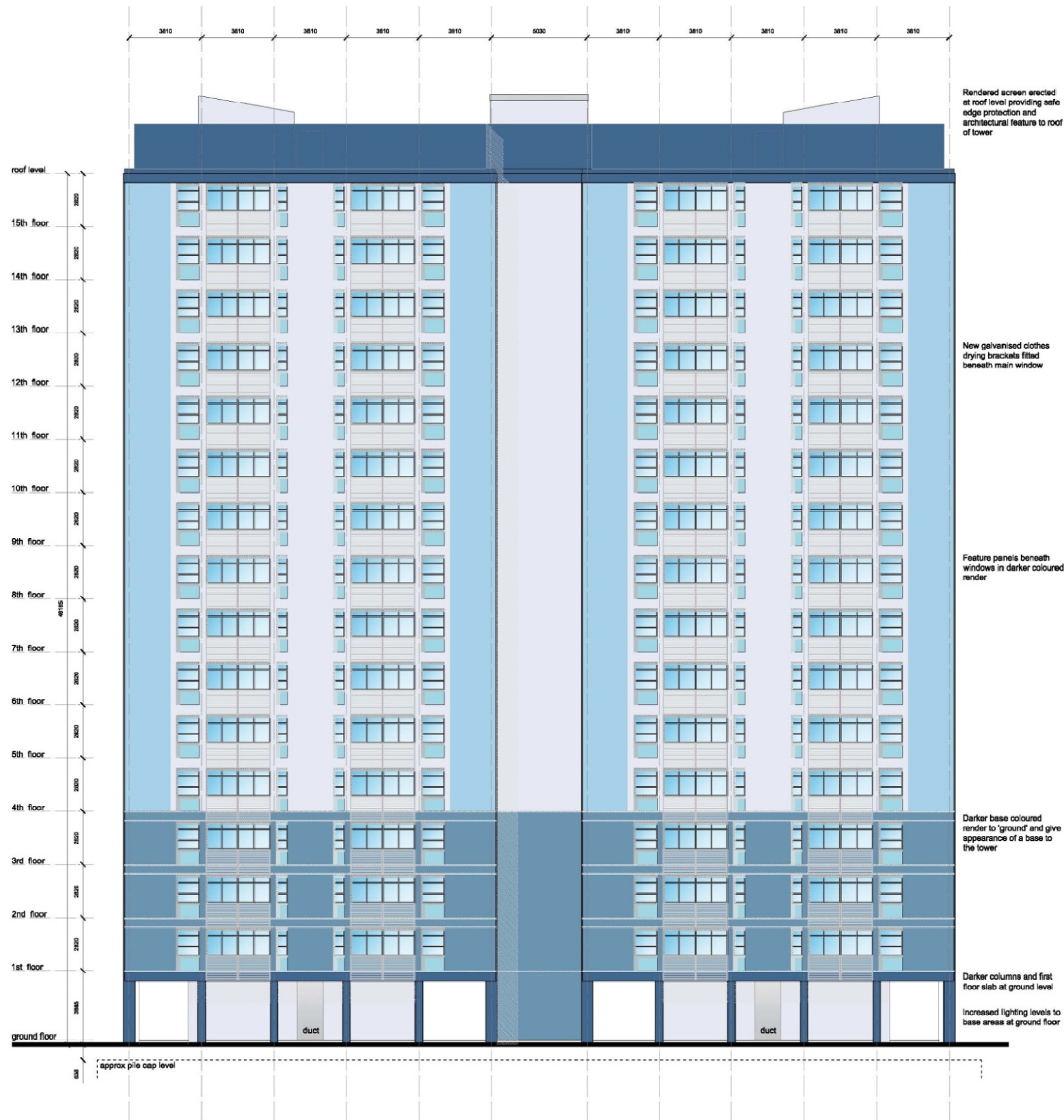
TYPICAL FRONT ELEVATION
